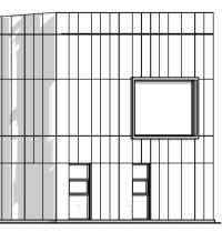
02.Brickwork Cream / Buff multi clay facing brick. Natural colour mortar Bucket handle joint. 03.**Extruded Aluminium Plank** Material: Aluminium
